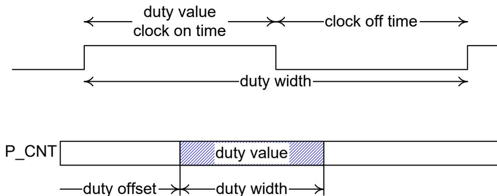
**Figure 8-37 Throttling Example**
