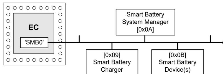
**Figure 13-70 Smart Battery Subsystem Devices**
