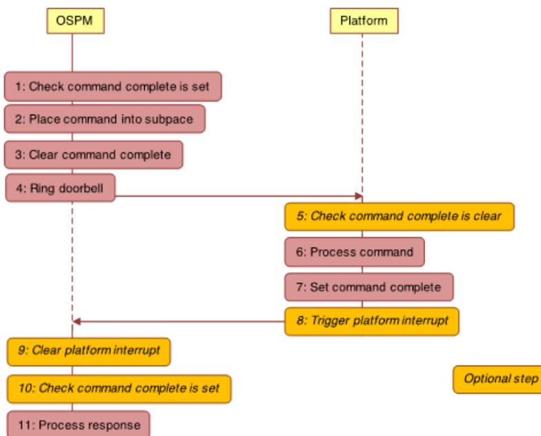
**Figure 14-72 Communication flow of the doorbell protocol**
