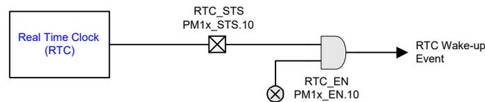
**Figure 4-11 RTC Alarm**
