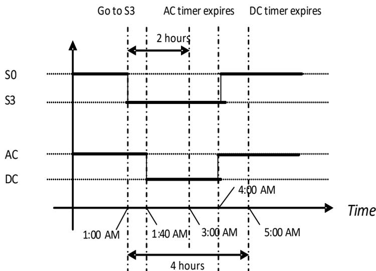
**Figure 9-53 System transitions with WakeAlarm -- Policy**
