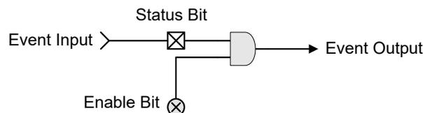
**Figure 4-4 Block Diagram of a Status/Enable Cell**
