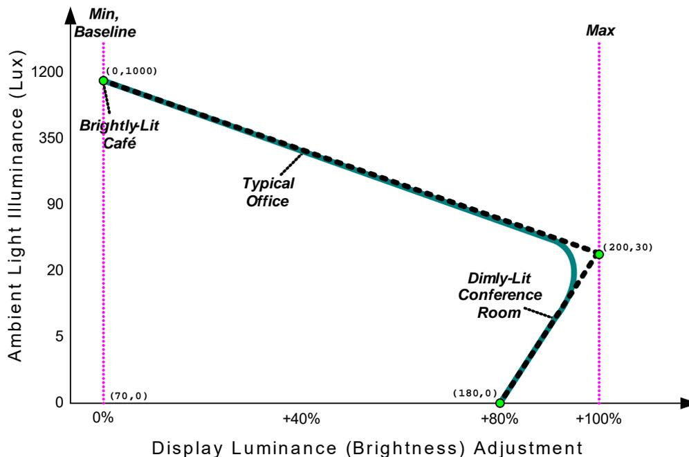
**Figure 9-49 Example Response Curve for a Transfective Display**
