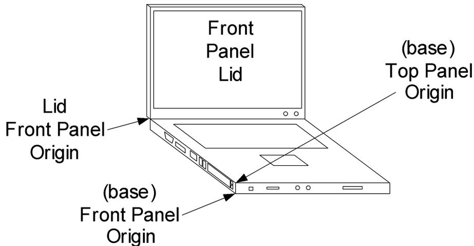
Fig. 6.2: Laptop Panel and Panel Origin Positions
