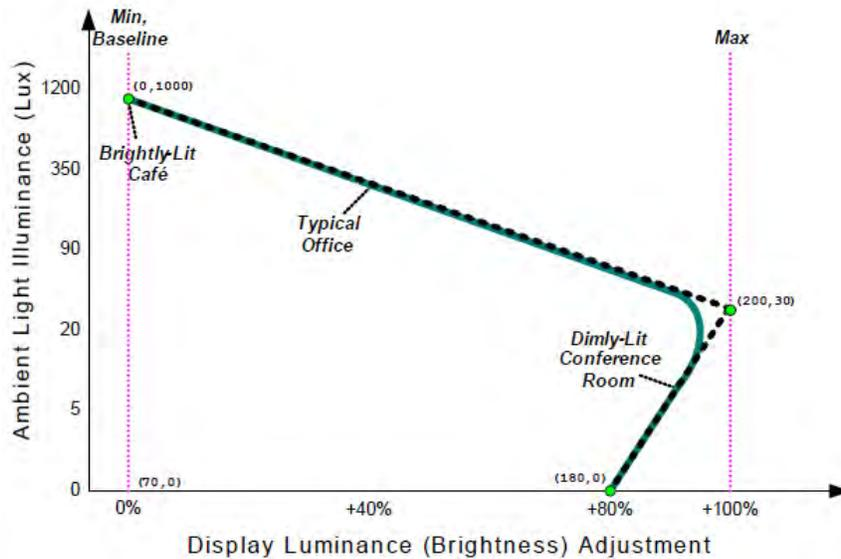
Fig. 9.3: Example Response Curve for a Transflective Display
