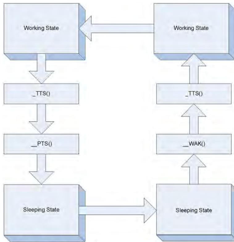
Fig. 7.1: Working / Sleeping State object evaluation flow
