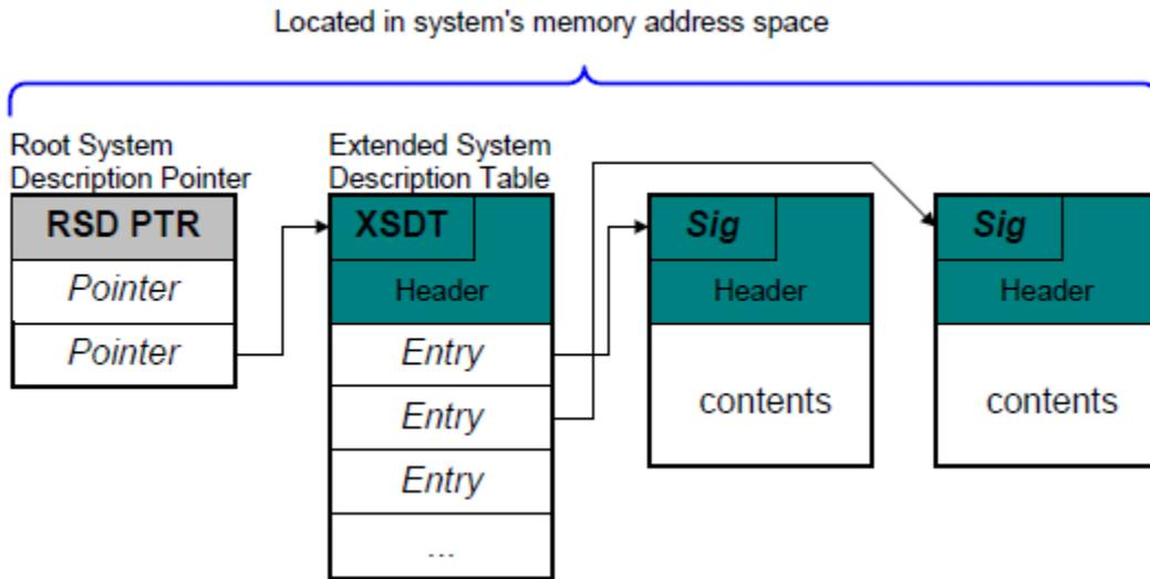
Fig. 5.1: Root System Description Pointer and Table
