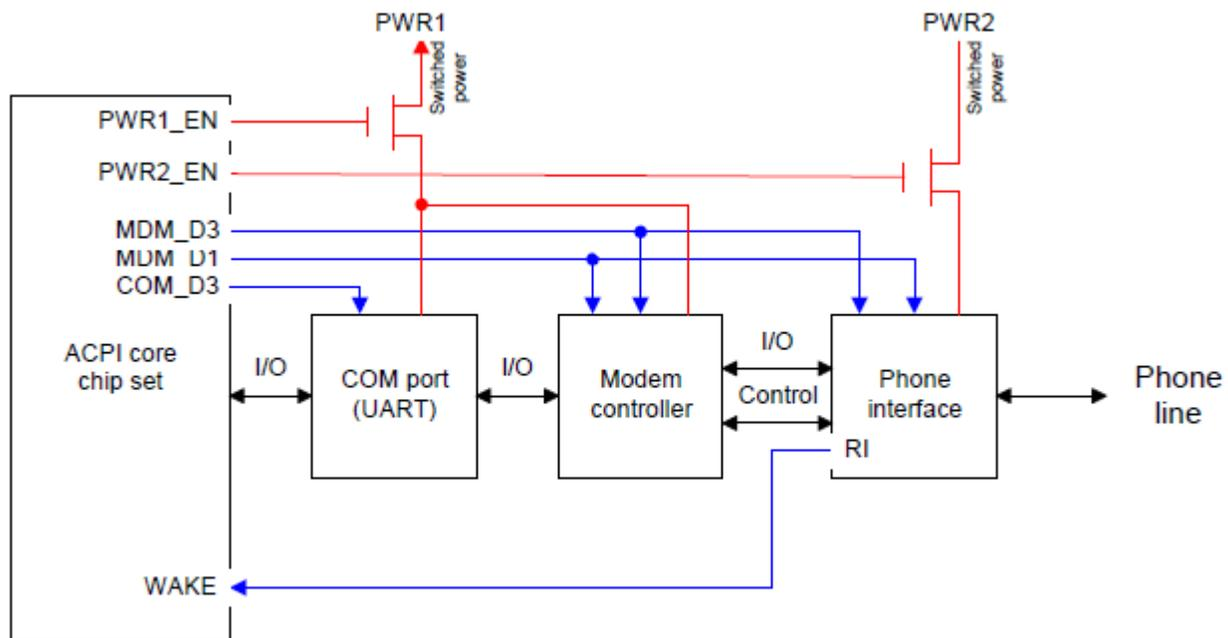
Fig. 3.2: Example Modem and COM Port Hardware
