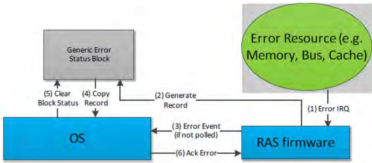
Fig. 18.1: APEI error flow example with external RAS controller
