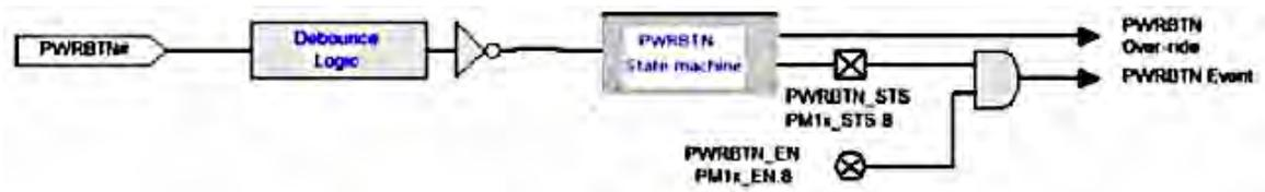
Fig. 4.8: Fixed Power Button Logic
