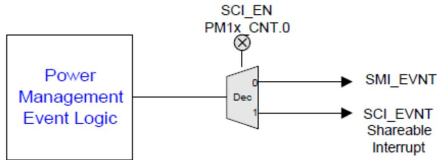
Fig. 4.12: Power Management Events to SMI/SCI Control Logic
