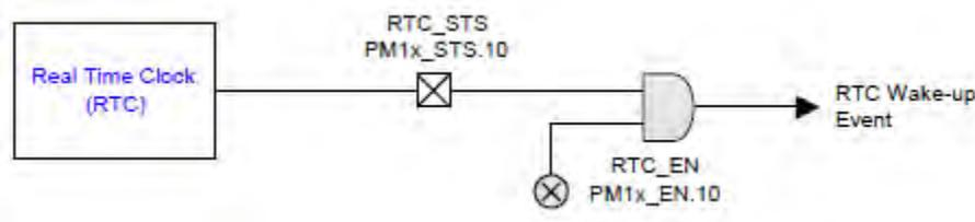
Fig. 4.11: RTC Alarm
