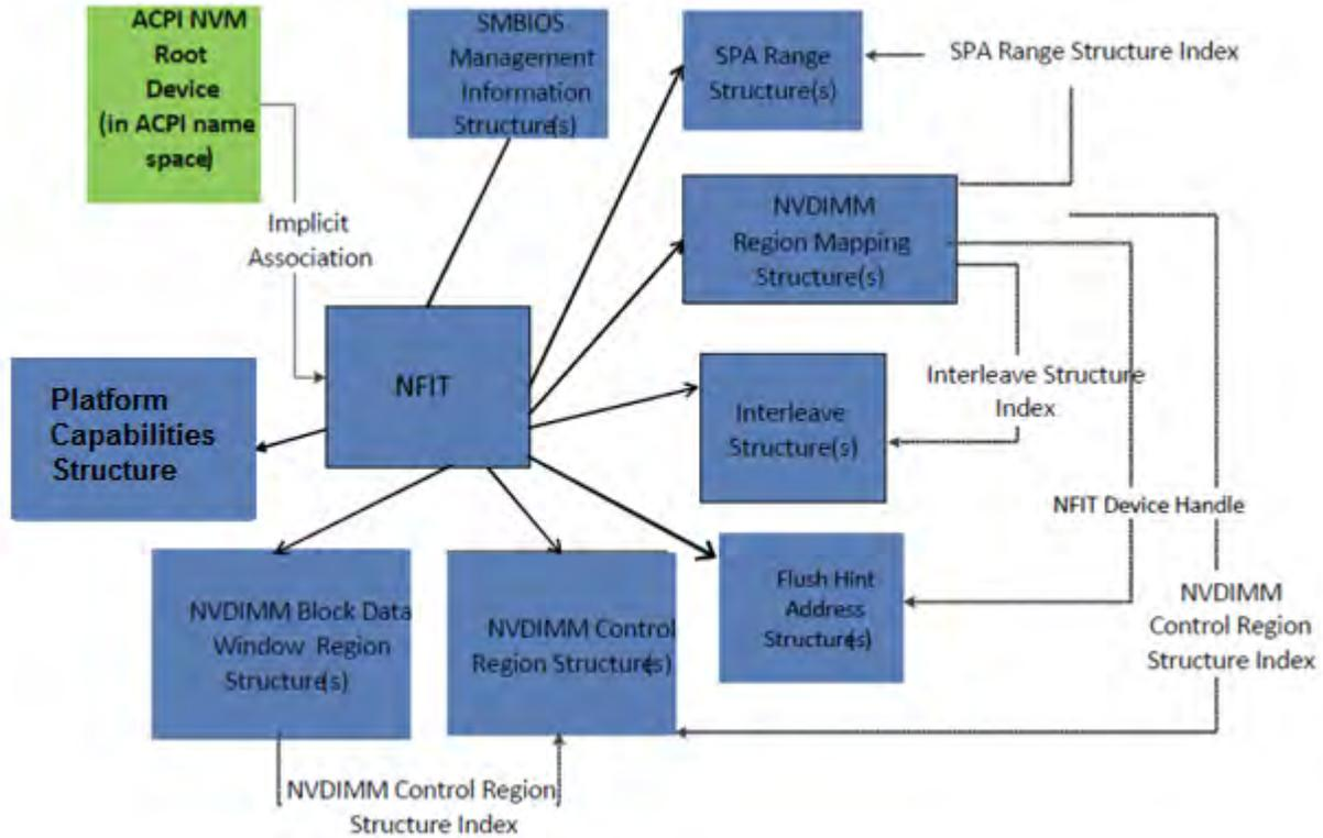
Fig. 5.9: NVDIMM Firmware Interface Table (NFIT) Overview
