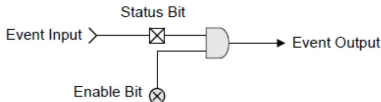
Fig. 4.4: Block Diagram of a Status/Enable Cell
