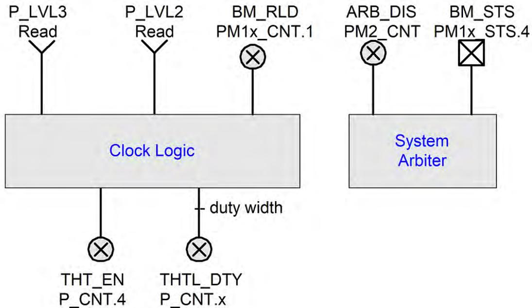
Fig. 8.5: ACPI Clock Logic (One per Processor)
