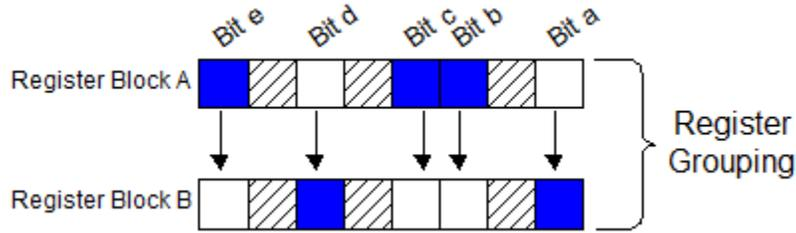
Fig. 4.5: Example Fixed Hardware Feature Register Grouping
