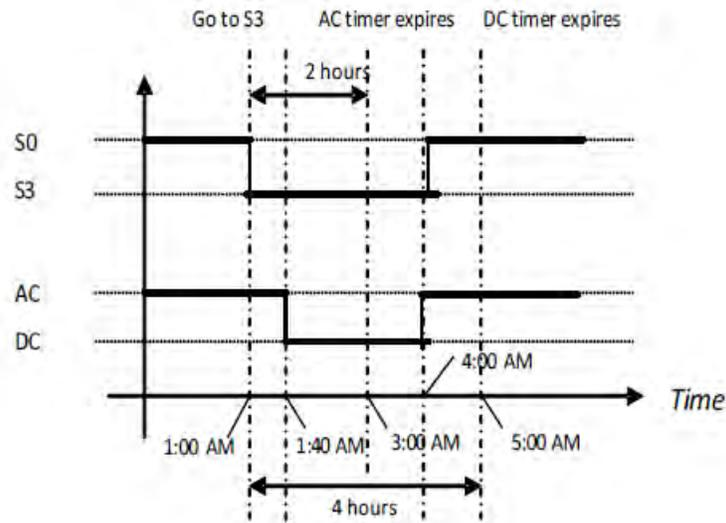
Fig. 9.7: System transitions with WakeAlarm — Policy
