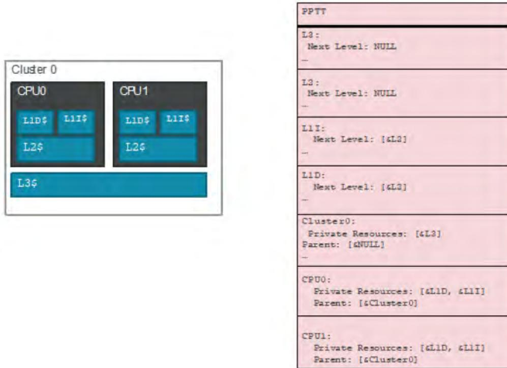
Fig. 5.15: Cache Type Structure - Type 1 Example
