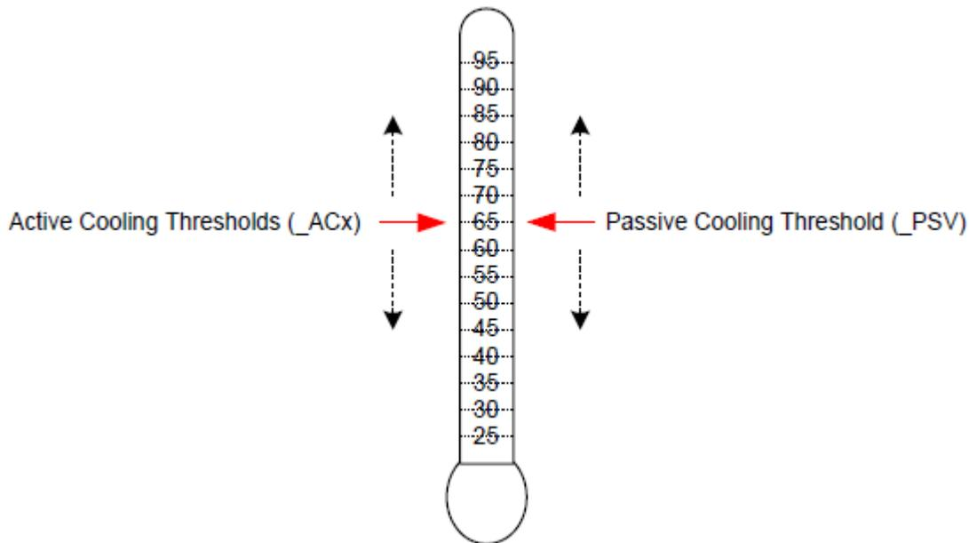
Fig. 11.4: Active and Passive Threshold Values
