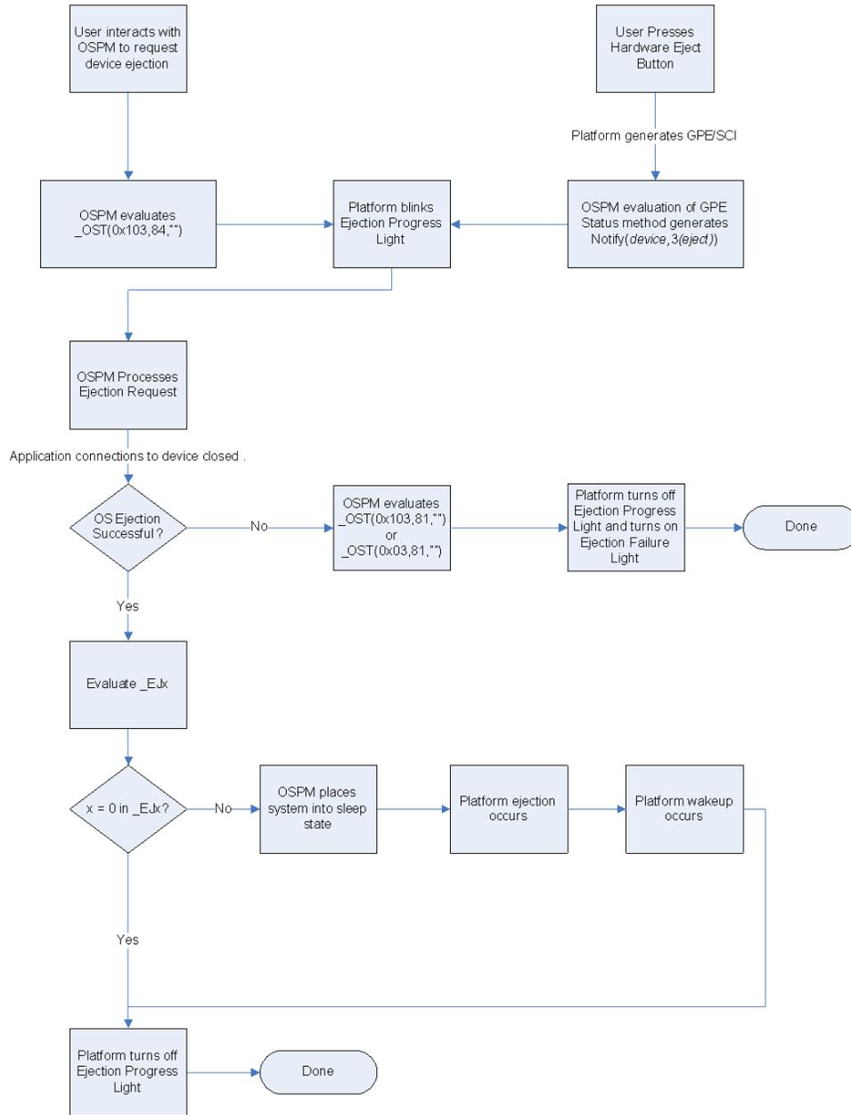
Fig. 6.6: Device Ejection Flow Example Using `_OST`
