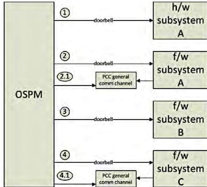
Fig. 5.13: Example: Platform with four debug triggers
