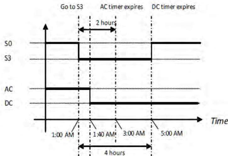
Fig. 9.6: System transitions with WakeAlarm — Timer
