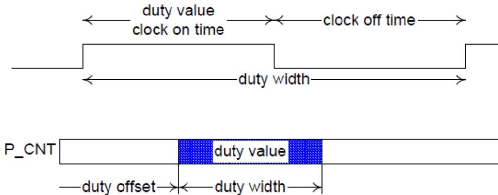
Fig. 8.2: Throttling Example
