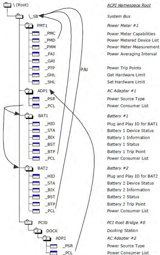
Fig. 10.6: Power Meter and Power Source/Docking Namespace Example
