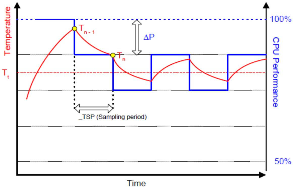
Fig. 11.3: Temperature and CPU Performance Versus Time
