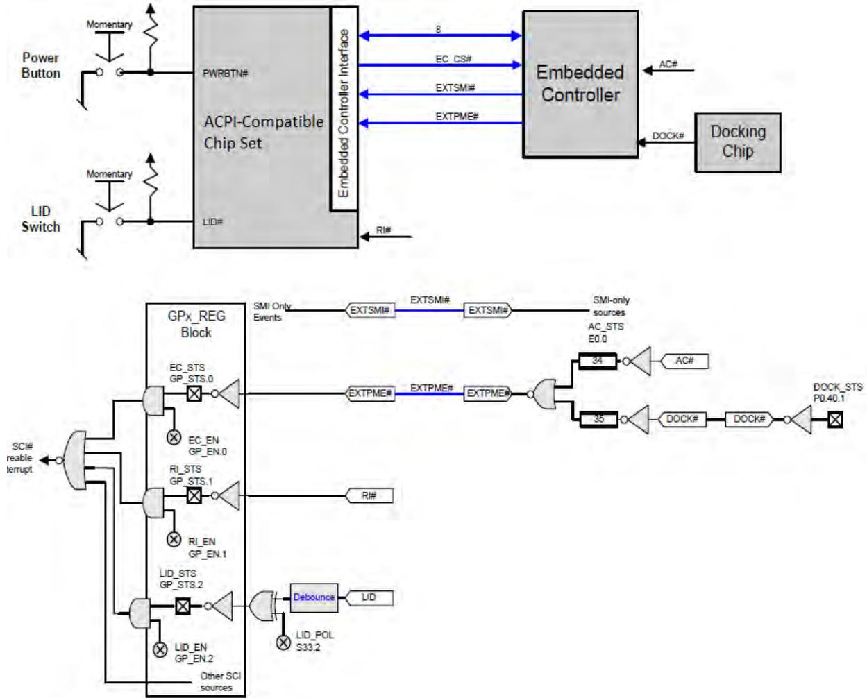
Fig. 4.13: Example of General-Purpose vs. Generic Hardware Events
